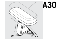
A30 Three Way Adjustable Arm Featuring Height Adjustment, Slides Forward or Rearward. Pad Also Shifts Inward and Outward for Width Adjustment.
